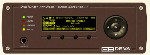
RF signal strength. BandScans are possible within any section of Band III, whereas the generated spectrum diagram shows the RF Level vs. the channels. Another great asset to this tool is the Loudness meter, which can be shown as defined by ITU BS.1770-4 and EBU R128 recommendations, as the product supports both.
