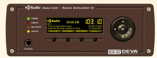
The Radio Explorer III HD Radio measures all important signal parameters, including the RF level, MPX deviation, Left & Right Audio levels values, as well as HD Radio® parameters such as DAAI and CDNR. Additionally, it boasts a Loudness meter, which can be shown as defined by ITU BS.1770-4 and EBU R128 recommendations, as the product supports both.
