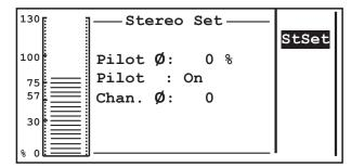
Pilot Add/remove pilot tone (convenient for some types of measurements). Chan.ph
