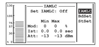
The IAMLC functionality provided by PTX-LCD adjusts the modulation level by adaptation of the input level, without the use of limitation or compression.
