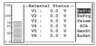
V1 Input voltage at pin 6 of REMOTE connector expressed in Volts (max 5 Volts).
