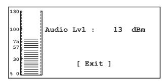
The level can be changed between -13 and +14 dBm, at 1 dB steps. On the back of the exciter there are the trimmers to perform fine regulations of the input levels.
