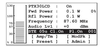
To work on a menu item, turn the encoder to select it and then push the encoder. Depending on the item, it could be possible that a new window is opened or that it will be possible to directly modify the parameter.
