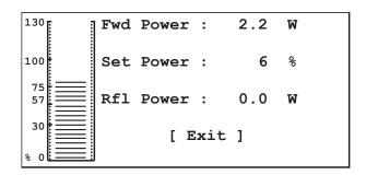
Output power reading and setting. The power reading is expressed in Watt, while the setting is expressed as percentage of the maximum output power. Pushing the encoder when the cursor is on this item will put you through the menu that permits to modify the power setting.
