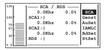
The PTX-LCD has three subcarrier transmission inputs named SCA1, SCA2 and RDS. This menu shows the modulation level achieved by each input both in kHz and in percent.
