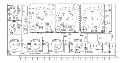
After the necessary elaboration (filtering, level adjustment, selection), the audio input section passes the signals on to the audio mainboard, that routes them to the coder card.
