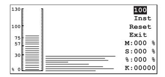
This graphic gives a visualization of the distibution af peak modulation levels. With this graphic, you can get a good idea of the modulation level reached during the working time.
