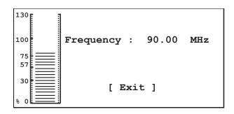
After choosing a new frequency value, the management software will ask you to confirm it (Are you sure... Yes/No). After confirmation pushing the encoder on the choice Yes, the exciter unlocks from the current frequency (the unlock LED is lit) and then locks again on the new frequency.
