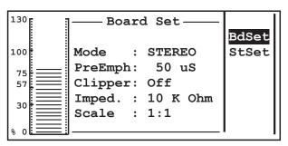
Mode Transmission mode selector: MONO, MPX\_U (unbalanced MPX BNC input), MBX\_B (balanced MPX XLR input), STEREO. The latter option is only enabled on the version with stereo coder.
