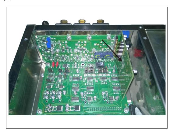
After the necessary elaboration (filtering, level adjustments, D/A conversion, selection), the audio input passes the signal on to the mainboard that routes it to the coder card.
