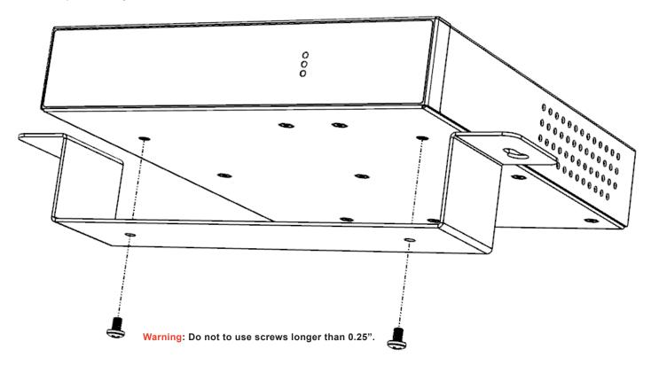
Note: The 1/2 U Surface Mount Bracket was designed to accommodate size 10 wood screws.
