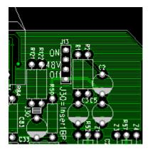
Figure 13: Triple Dig Module Phantom Power Jumper settings
