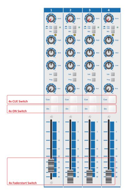
Figure 2. USB Channel Controls
