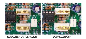
Figure 8: Triple Module EQ Jumper settings
