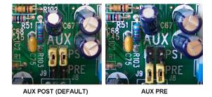
Figure 17: Telco Module AUX Jumper settings
