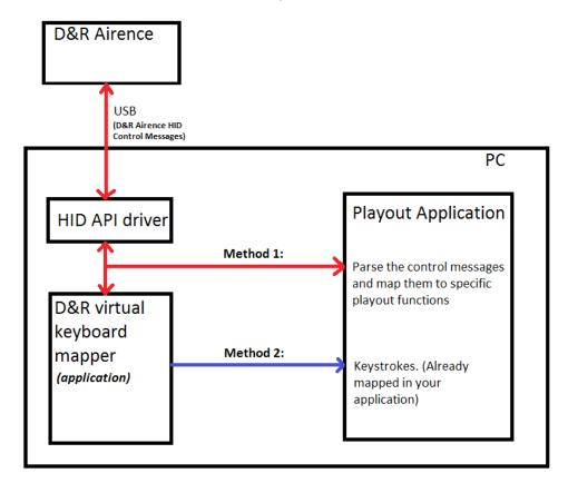
Figure 3. Airlab(Airence) control methodologies
