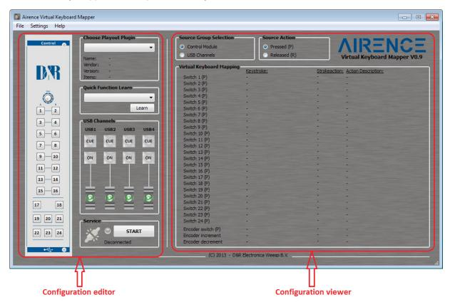
Figure 4. Airlab/Airence virtual keyboard mapper, Windows-based application
