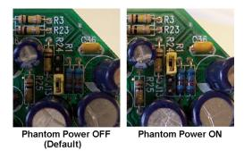
Figure 7: Triple Module Phantom Power Jumper settings
