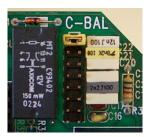
Figure 18: Telco Module C-Balance Setting
