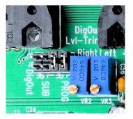
Figure 14: Triple Dig Module Digital Output Select Jumper and Digital Output Level trim
