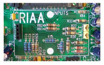
Figure 9: R.I.A.A connection on Triple module
