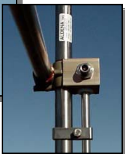
Dipolo a Gamma-match. Gamma-match type dipole.
